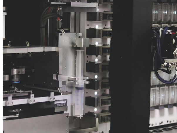
P1000: slide scanner with microscope ( left ) with sample storage and robot arm ( right )
