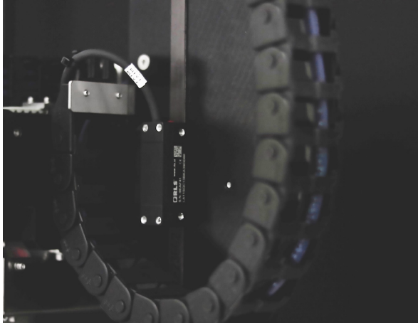
LA11 magnetic encoder in-situ on the robot arm
