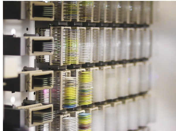
P1000 has capacity for 1000 slides and can digitise all of them in one work-shift
