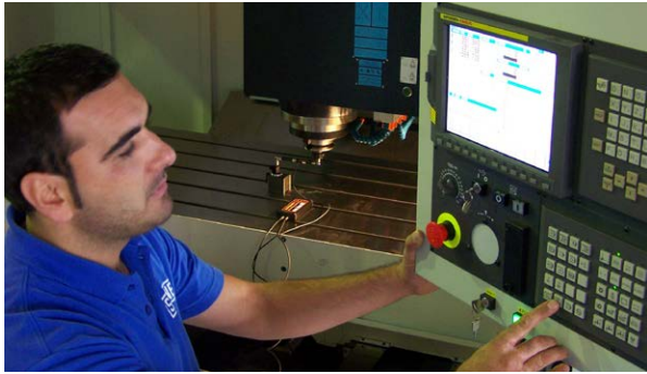
Spinner use the ballbar to set up the control systems at the factory, then to help mechanically adjust out geometry errors caused by installation at a customer's site
