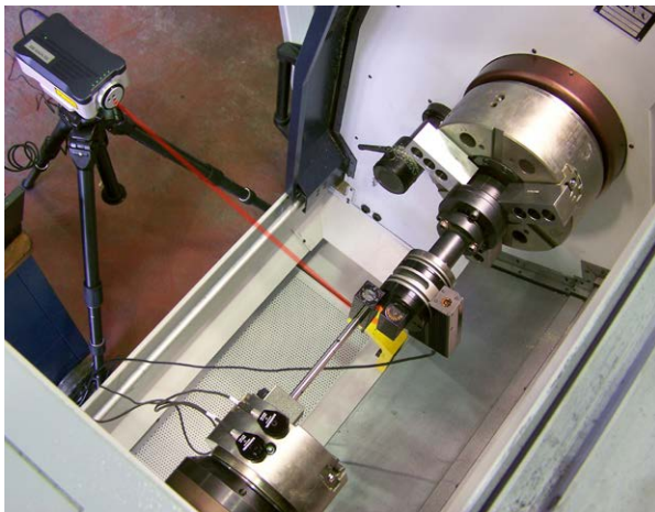
Calibration of a turning centre sub-spindle using the Renishaw RX10 rotary calibrator
