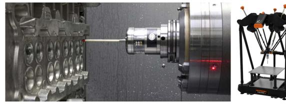
Renishaw OMP60 optical transmission probe measuring key engine features
