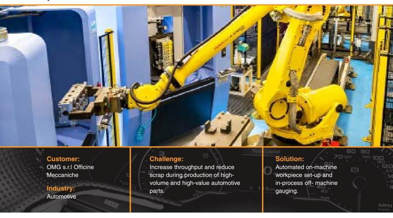
An increase in production orders for new breeds of high-volume and high-value automotive components required OMG to consider alternative approaches to part inspection. Investments in off-machine gauging and on-machine probing enabled the company to increase manufacturing throughput, avoid rejects and reduce scrap.
